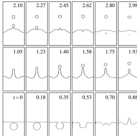
FIGURE 17. Evolution of a water jet resulting from a submerged gas bubble.  $\lambda = 0.001$ ,  $\eta = 0.01$ ,  $Re = 474$ ,  $We = 1$ , and  $Fr = 0.64$ . This corresponds to an air bubble of radius 4 mm in water.
