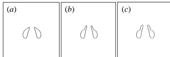
FIGURE 13. Comparison for various Reynolds numbers for the rising gas bubble problem with  $\lambda = 0.001$ ,  $\eta = 0.01$ ,  $B = 200$ , and  $Fr = 1$  at  $t = 2.0$ . (a)  $Re = 100$ , (b)  $Re = 400$ , (c)  $Re = \infty$ .
