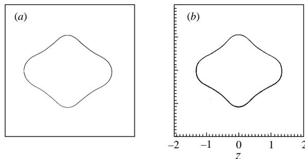
FIGURE 3. Comparison at  $t = 1.1$  of the motion of an oscillating viscous drop in zero gravity computed using the level set method (a) and computed using the boundary integral method (b) of Lundgren & Mansour (1988). The drop is initialized with a  $P_4$  shape with  $\lambda = 0.01$ ,  $\eta = 0.01$ ,  $Re = 2000$ ,  $We = 2$ , and  $Fr = \infty$ .
