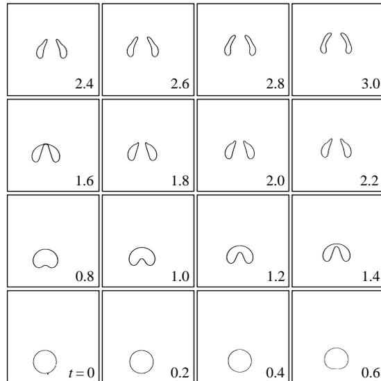
FIGURE 11. Evolution of an initially spherical gas bubble with  $\lambda = 0.001$ ,  $\eta = 0.01$ ,  $Re = 100$ ,  $B = 200$ , and  $Fr = 1$ .
