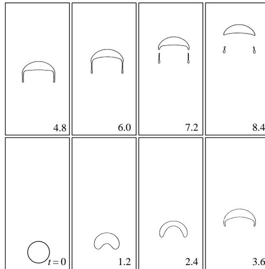
FIGURE 6. Evolution of a viscous gas bubble with  $\lambda = 0.0011$ ,  $\eta = 0.0085$ ,  $Re = 24.4$ ,  $We = 27.2$ , and  $Fr = 0.88$ . This corresponds to bubble C of table I in Hnat & Buckmaster (1976).
