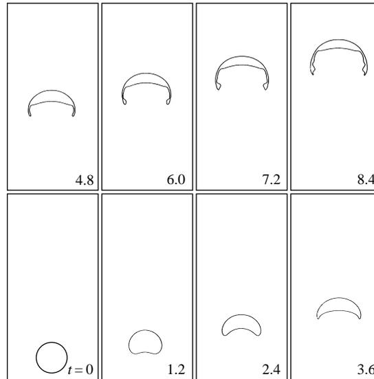
FIGURE 8. Evolution of a viscous gas bubble with  $\lambda = 0.0011$ ,  $\eta = 0.0085$ ,  $Re = 70$ ,  $We = 115$ , and  $Fr = 0.99$ . The initial data for this problem are the result at  $t = 4.0$  of allowing a bubble to rise with the parameters of bubble A and then varying  $Re$ ,  $We$ , and  $Fr$  linearly until they reach the parameters given above at  $t = 4.0$ .
