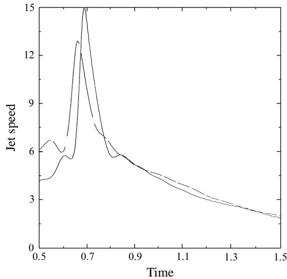
FIGURE 19. The jet speed for figures 17 and 18. The solid line is for the 4 mm bubble and the dashed line is for the 5 mm bubble.
