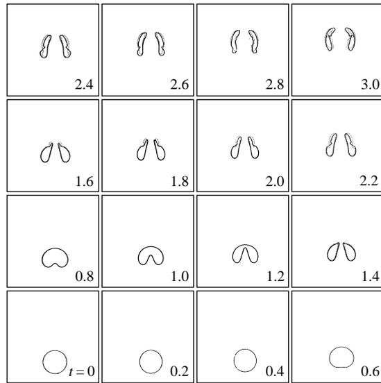
FIGURE 9. Evolution of an initially spherical gas bubble with  $\lambda = 0.001$ ,  $Re = \infty$ ,  $B = 200$  and  $Fr = 1$ . The dashed lines represent the results from the boundary integral scheme and the solid lines represent the results from the level set method.
