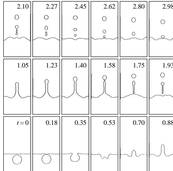
FIGURE 18. Evolution of a water jet resulting from a submerged gas bubble.  $\lambda = 0.001$ ,  $\eta = 0.01$ ,  $Re = 531$ ,  $We = 1$ , and  $Fr = 0.29$ . This corresponds to an air bubble of radius 5 mm in water.
