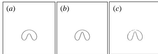
FIGURE 12. Comparison for various Reynolds numbers for the rising gas bubble problem with  $\lambda = 0.001$ ,  $\eta = 0.01$ ,  $B = 200$ , and  $Fr = 1$  at  $t = 1.2$ . (a)  $Re = 100$ , (b)  $Re = 400$ , (c)  $Re = \infty$ .
