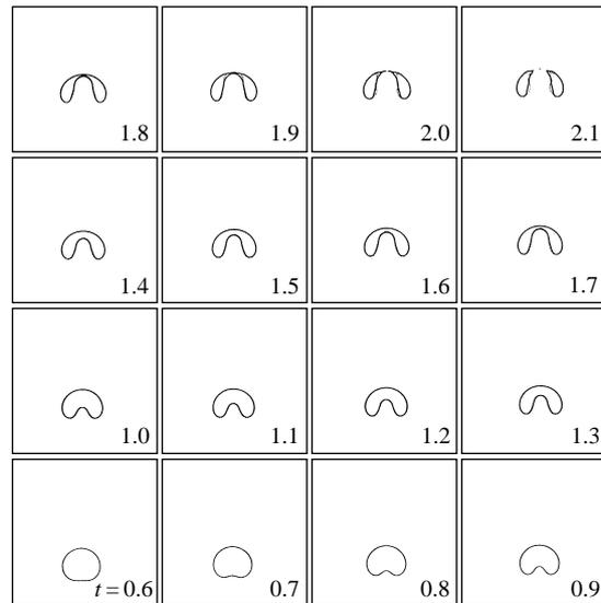
FIGURE 10. Evolution of an initially spherical gas bubble with  $\lambda = 0.001$ ,  $Re = \infty$ ,  $B = 10$  and  $Fr = 1$ . The dashed lines represent the results from the boundary integral scheme and the solid lines represent the results from the level set method.
