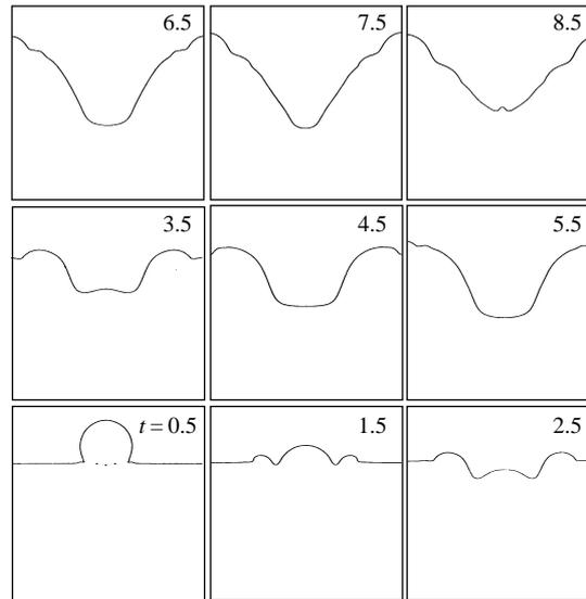
FIGURE 14. Evolution of a drop impinging on a water surface with  $\lambda = 0.001$ ,  $Re = \infty$ ,  $Fr = 26.12$ , and  $We = 21.95$ . This corresponds, approximately, to a 2.5 mm water drop hitting the water surface at  $0.8 \text{ m s}^{-1}$ .
