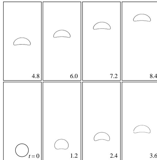
FIGURE 4. Evolution of a viscous gas bubble with  $\lambda = 0.0011$ ,  $\eta = 0.0085$ ,  $Re = 9.8$ ,  $We = 7.6$ , and  $Fr = 0.76$ . This corresponds to bubble A of table I in Hnat & Buckmaster (1976).
