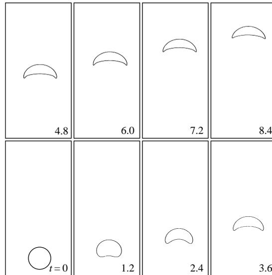
FIGURE 7. Evolution of a viscous gas bubble with  $\lambda = 0.0011$ ,  $\eta = 0.0085$ ,  $Re = 24.4$ ,  $We = 27.2$ , and  $Fr = 0.88$ . This corresponds to bubble C of table I in Hnat & Buckmaster(1976). The initial data for this problem are the result at  $t = 4.0$  of allowing a bubble to rise with the parameters of bubble A and then linearly varying  $Re$ ,  $We$ , and  $Fr$  until they reach the parameters of bubble C at  $t = 4.0$ .
