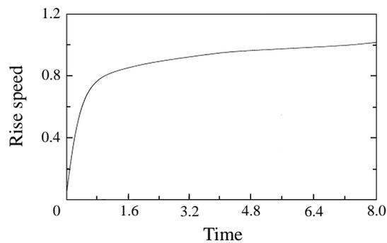
FIGURE 5. The time evolution of the velocity of the top of the bubble shown in figure 4.
