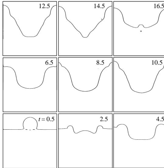
FIGURE 15. Evolution of a drop impinging on a water surface with  $\lambda = 0.001$ ,  $Re = \infty$ ,  $Fr = 58.77$ , and  $We = 49.38$ . This corresponds, approximately, to a 2.5 mm water drop hitting the water surface at  $1.2 \text{ m s}^{-1}$ .
