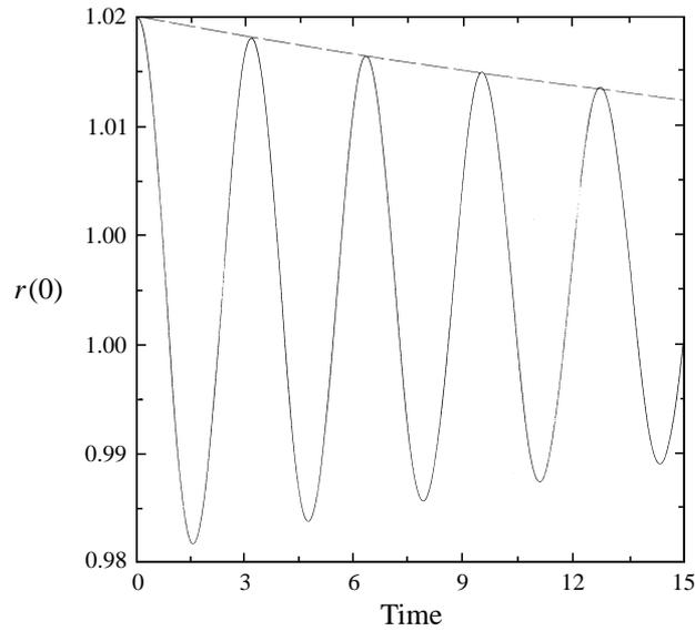
FIGURE 1. Motion of a viscous drop in zero gravity with  $\lambda = 0.01$ ,  $\eta = 0.01$ ,  $Re = 200$ ,  $We = 2$ , and  $Fr = \infty$ : the time evolution of  $r(0, t)$  initialized with  $P_2$  shape (the solid curve) along with the predicted viscous envelope (the dashed curve).
