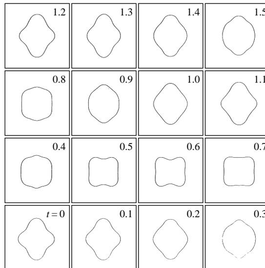
FIGURE 2. Motion of a viscous drop in zero gravity with  $\lambda = 0.01$ ,  $\eta = 0.01$ ,  $Re = 2000$ ,  $We = 2$ , and  $Fr = \infty$ : the shape oscillations when the drop is initialized with a  $P_4$  shape.
